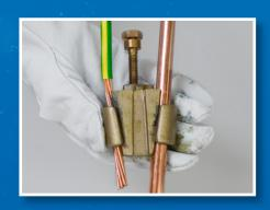
Ensuring placement is correct, the shear head bolt is tightened using a six sided hex spanner or socket until the correct torque is reached and the head shears off
