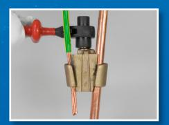
The connection is made correctly everytime due to the shear head bolt which pushes the wedge into place as it is tightened.
